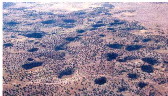
Figure 5. Aerial view of The Sinks, looking south down monoclinical flexure toward collapsed Dry Lake Valley (see Fig. 4). Sinkhole locations are strongly influenced by joint openings and collapse grabens in Coconino Sandstone. Nearly 50 sinkholes are shown in this one view, the largest being 100m across.
